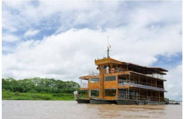
The M/V Delfin I is a three-deck, steel-hulled, trimaran river boat built in 1982 and completely refurbished in 2010. Due to her very shallow draft (4.5 feet), she provides travelers with a comfortable, yet adventurous way to visit the remote tributaries of the upper Amazon. Small motor launches take passengers on excursions to remote tributaries and lakes.
